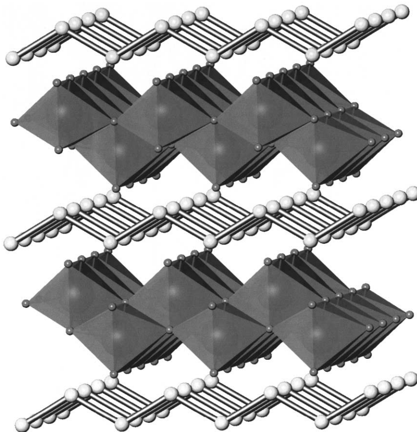
Fig. 10. Orthorhombic structure of \text{Ca}_2\text{AuN} . Infinite zig-zag chains of \text{Au}^- ions (medium spheres) alternate with corrugated [\text{Ca}_2\text{N}]^+ layers of edge-sharing \text{NCa}_6 octahedra along the b -axis.
